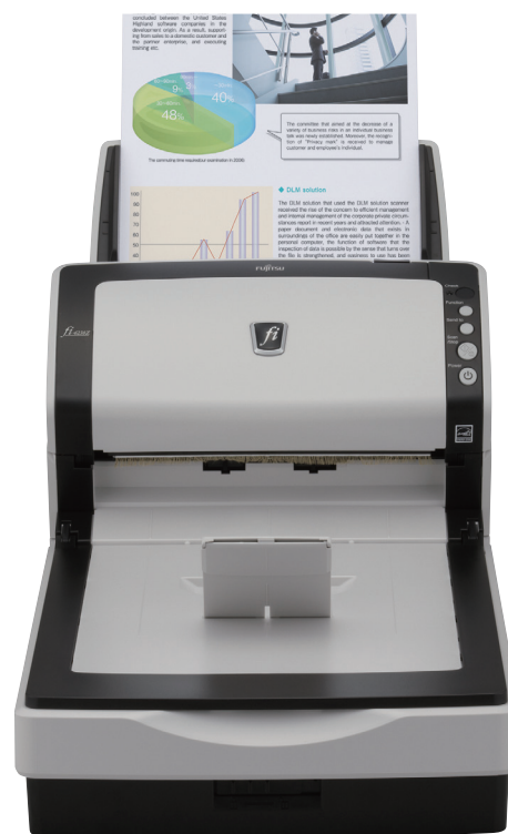
Fujitsu's new scanners offer a post imprinter option that prints identification markers like dates, alphanumeric codes and symbols on the reverse side of the original document. This makes it easier to locate the original scanned document when needed for reference.
