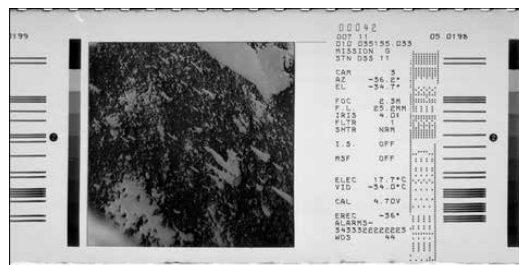
Another example of a Surveyor mission film image captured by a 70-mm film camera and photographed onto special recording film.
