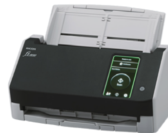
Fi-8040 – Entry Level 40 Page a Minute A4 Desktop Scanner with LAN and USB Connection
